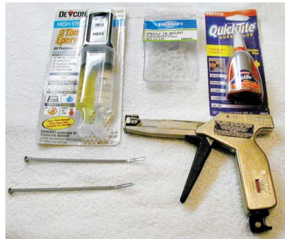
Figure 6. Shell repair materials.
